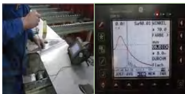
臂架100%UT探伤 100% UT flaw detection for boom
