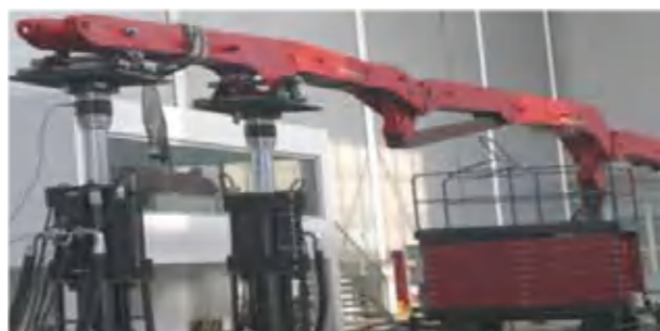
臂架结构破坏性测试 Destructive test of boom structure
